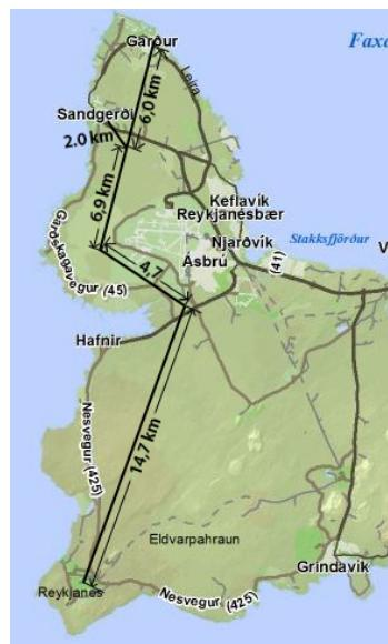
Figure 3.4: Pipeline from RPP to Skinnfiskur and Nesfiskur [Map taken from [www.ja.is](http://www.ja.is)].
