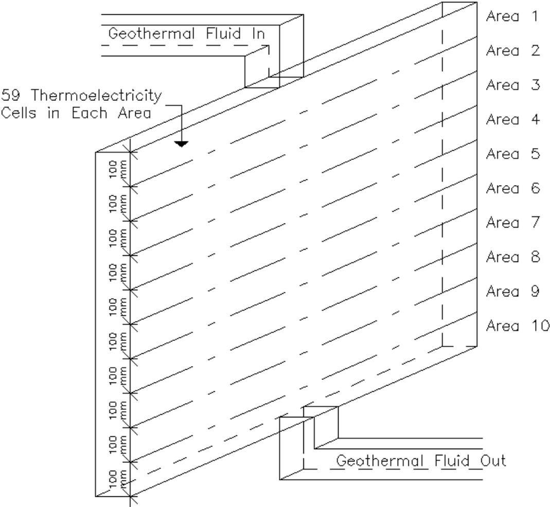
**Figure 23 Drawing describing the geometry for one square meter of thermoelectricity device**
