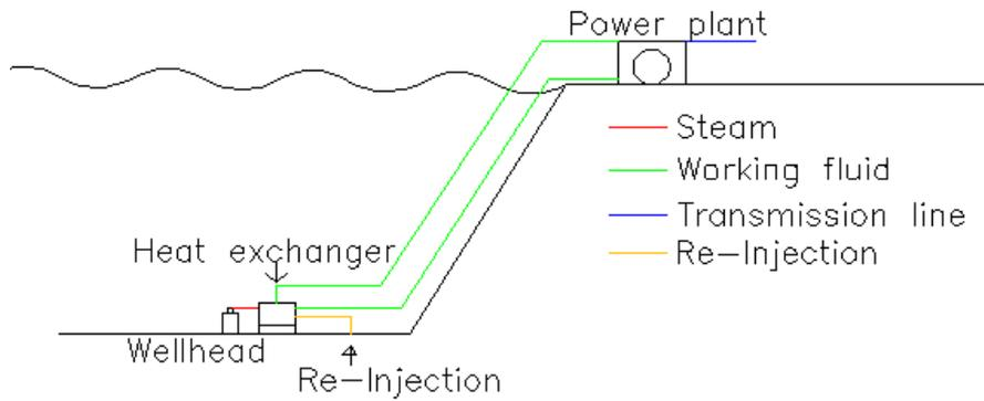
**Figure 29 Binary power plant based on land**
