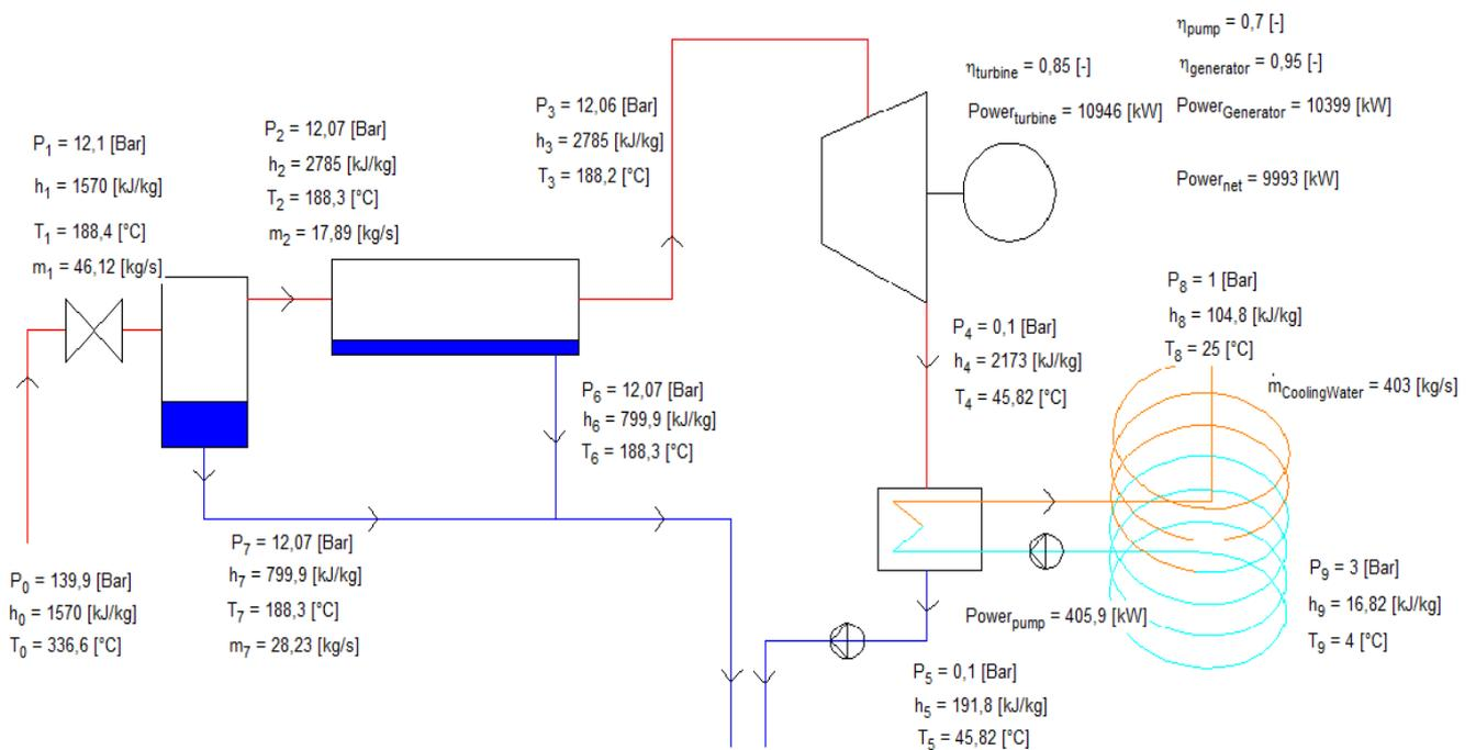
**Figure 25 Diagram drawing for single flash on a platform with components placed in their position**
