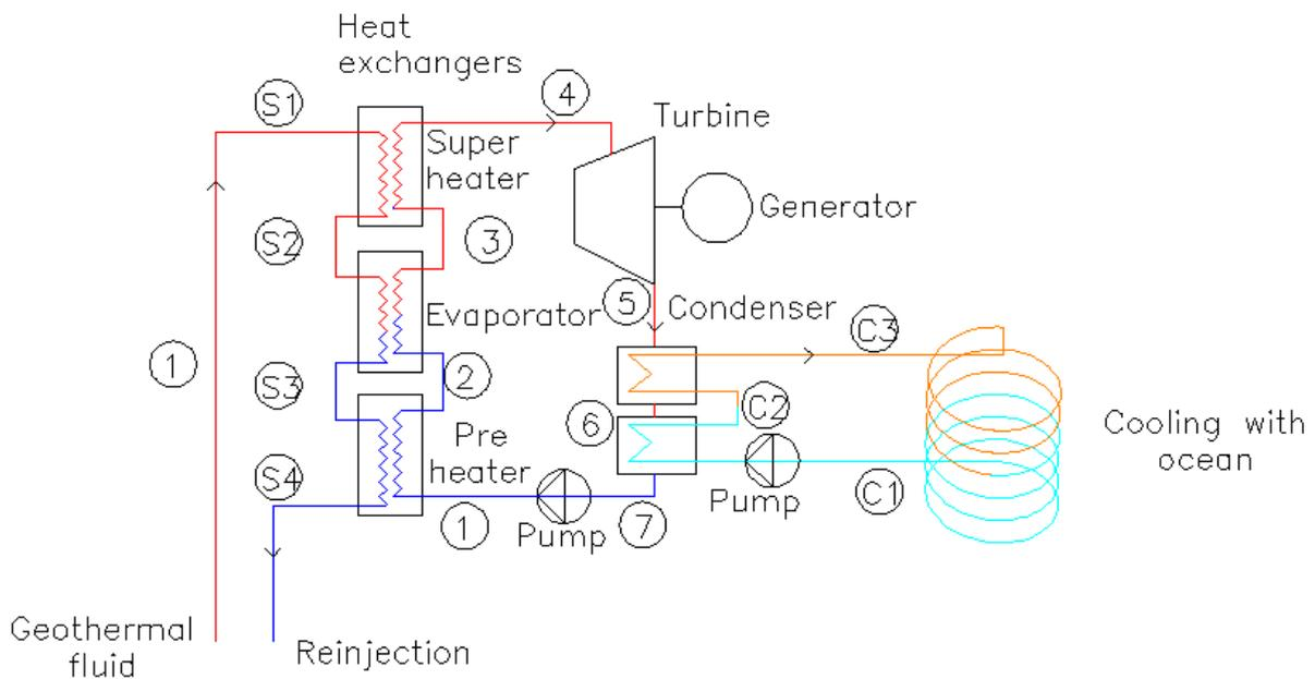
**Figure 19** Process diagram of a binary cycle
