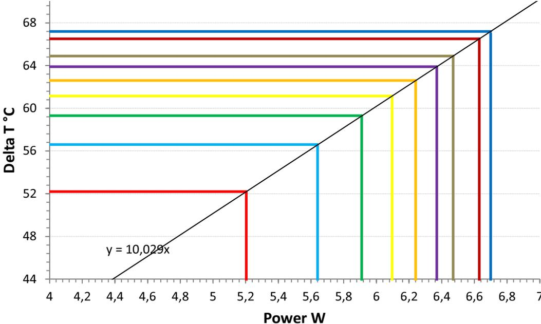
Figure 34 Regression graph showing power for one cell for given ΔT
