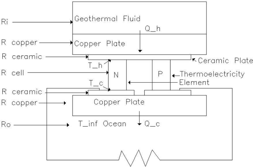
Figure 21 Single thermoelectric couple
