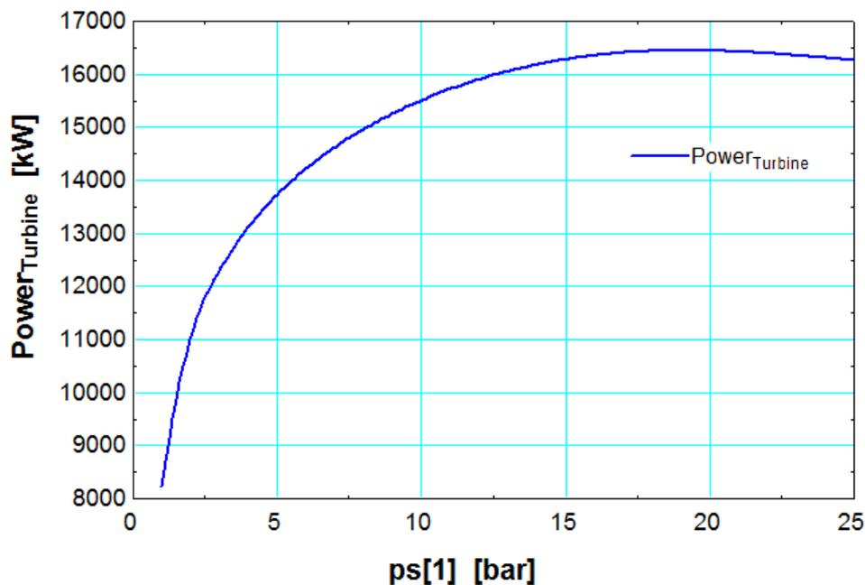
**Figure 30 Plot power – pressure of geothermal liquid in binary cycle**
