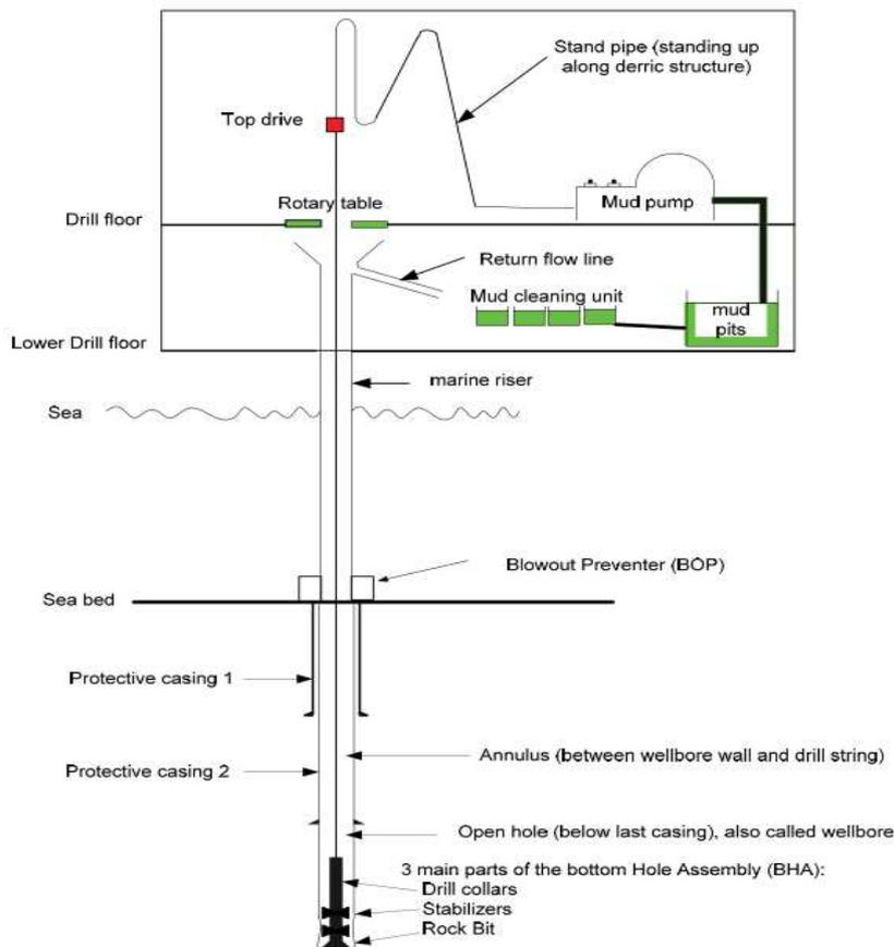
Figure 10 Offshore drilling process circle [14]
