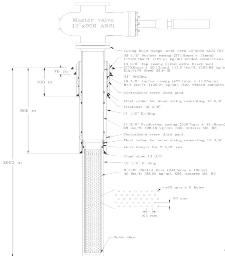
Figure 11 Geothermal casing design [15]
