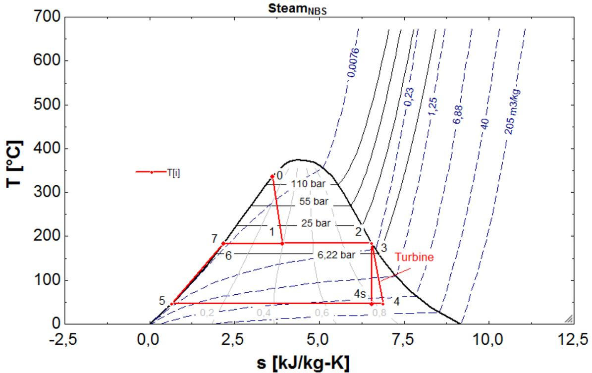
Figure 18 Temperature - entropy diagram for single flash
