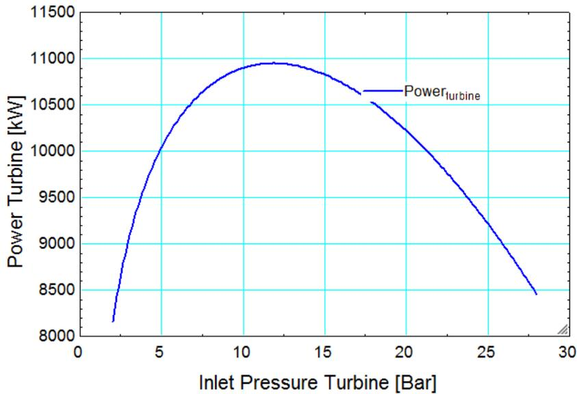
Figure 26 Plot power - pressure for single flash on platform
