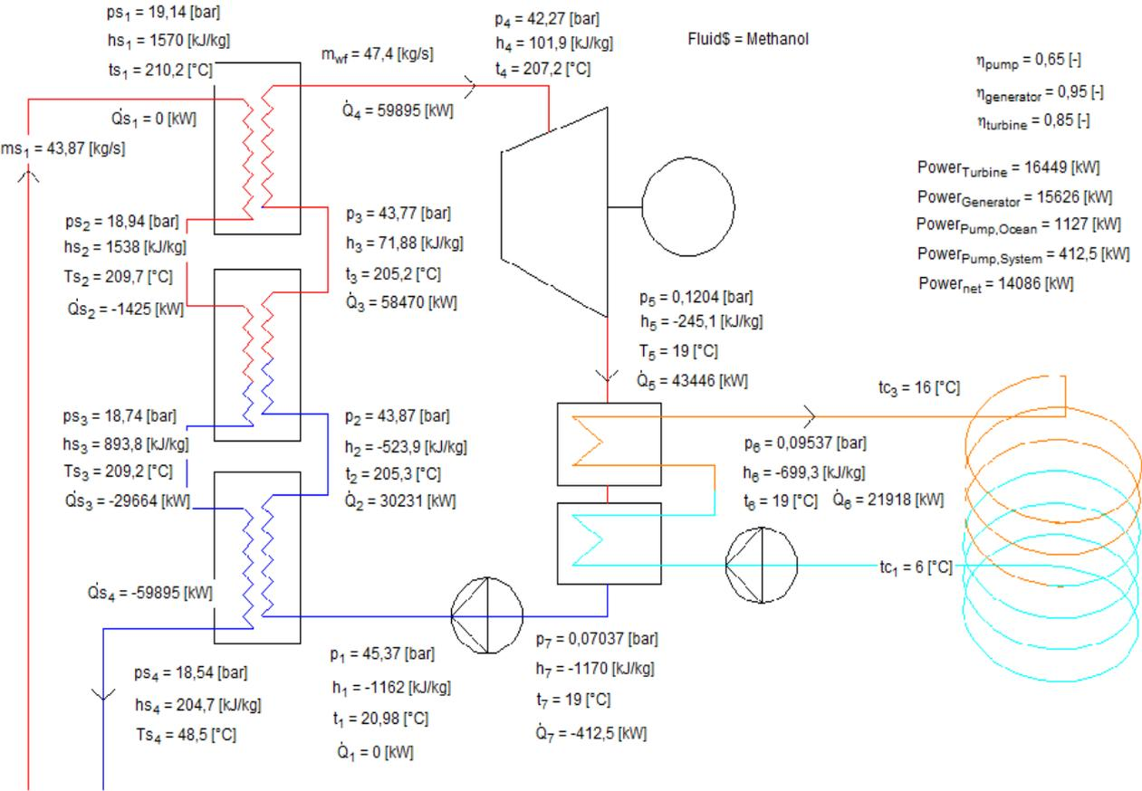
Figure 31 Process diagram of a binary cycle showing the conditions for each state
