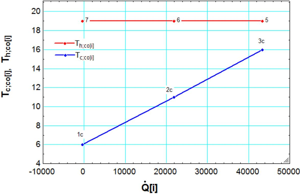
Figure 33 The condenser showing how the heat is rejected from the condensing working fluid to the cooling fluid
