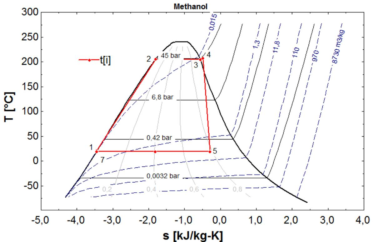
Figure 20 Temperature - entropy diagram for binary cycle calculation with methanol as the working fluid
