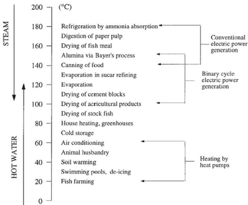
Figure 17 Líndal diagram showing utilization of geothermal energy at different temperatures [23]
