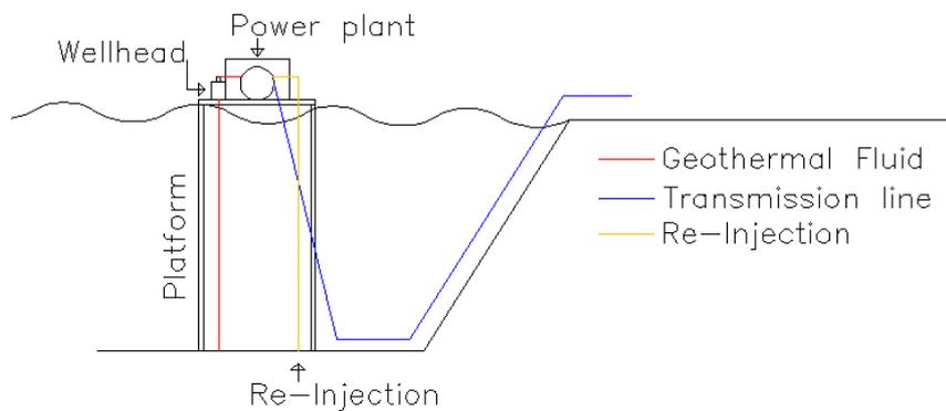
Figure 24 Platform based power plant
