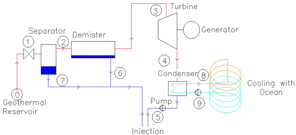
**Figure 16** Process diagram of a single flash cycle
