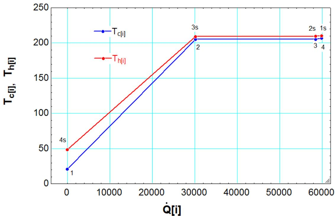
Figure 32 The heat exchange process showing how the heat is transferred from the geo-fluid to the working fluid
