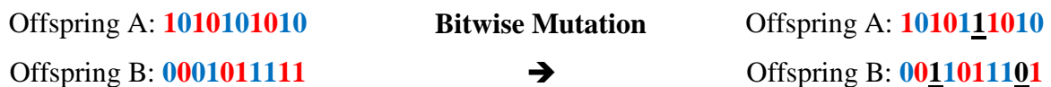
Figure 11: Example of two 10 bit chromosomes undergoing bitwise mutation (black, underlined bits are those that were altered by bitwise mutation). The mutation of Offspring A has no effect on the mutation of Offspring B.
