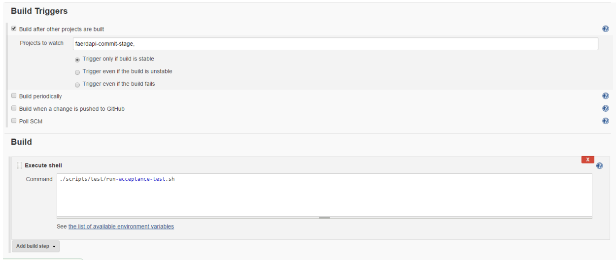
Figure 14: Jenkins configuration for faerdapi-acceptance-stage
