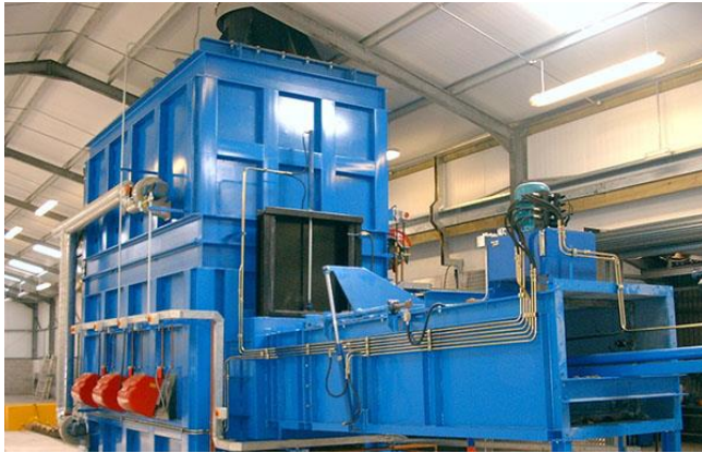
Figure 3.2 Stepped hearth IED/WID incinerator Source: Matthews Environmental Solutions Ltd (2021)
