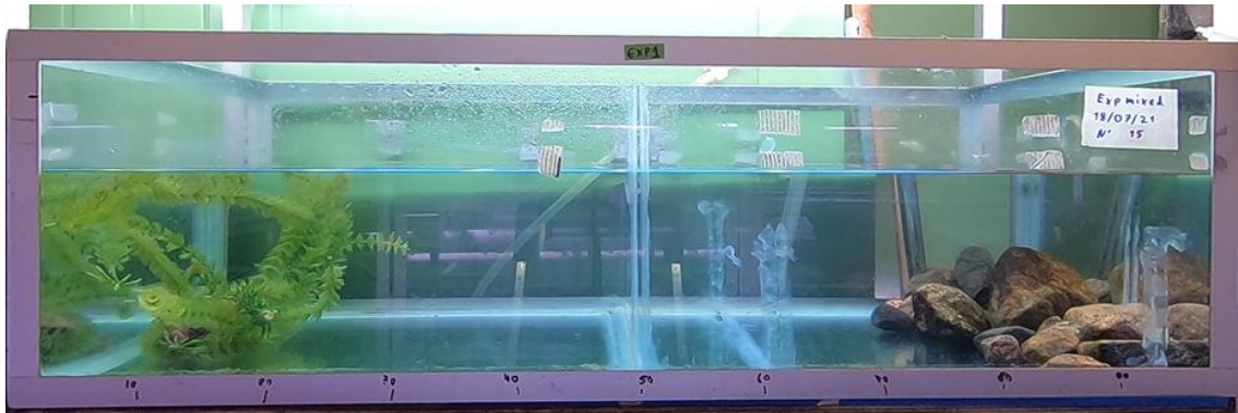
Figure 5. Example of an experimental tank used for the behavioural study. In this case it is the mixed tank, where the two elements used in the study can be observed. On the left side there is vegetation and on the right side there are rocks.
