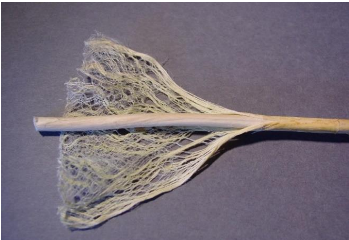
Figure 5 Hemp stem subjected to retting (decomposition of the softer tissues). The fibre in the top portion has been separated from the woody core. Photo by Natrij, released into the public domain (Natrij, 2011).
