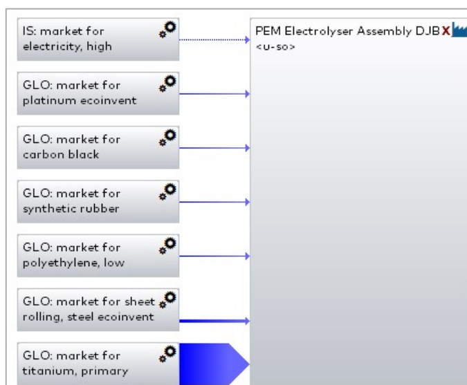
Figure 12: GaBi model for the Assembly of PEM Electrolyser in Iceland using LCI data from Table 4
