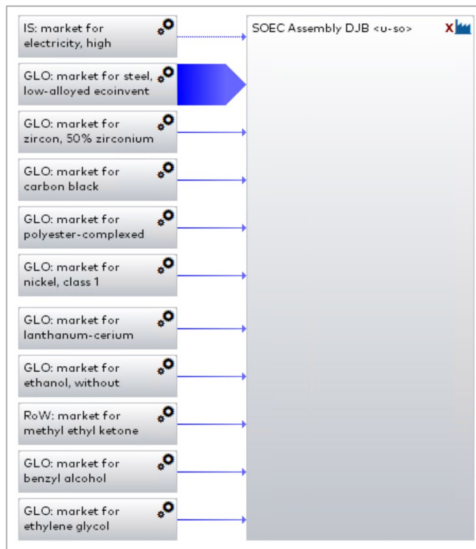
Figure 14: GaBi model for the Assembly of a 1 MW SOEC in Iceland using LCI data from Table 6
