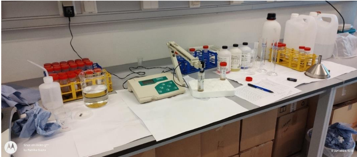
Figure 2.8 Soil pH(water) measurement setup (Photo by Parnika Gupta, 2022).
