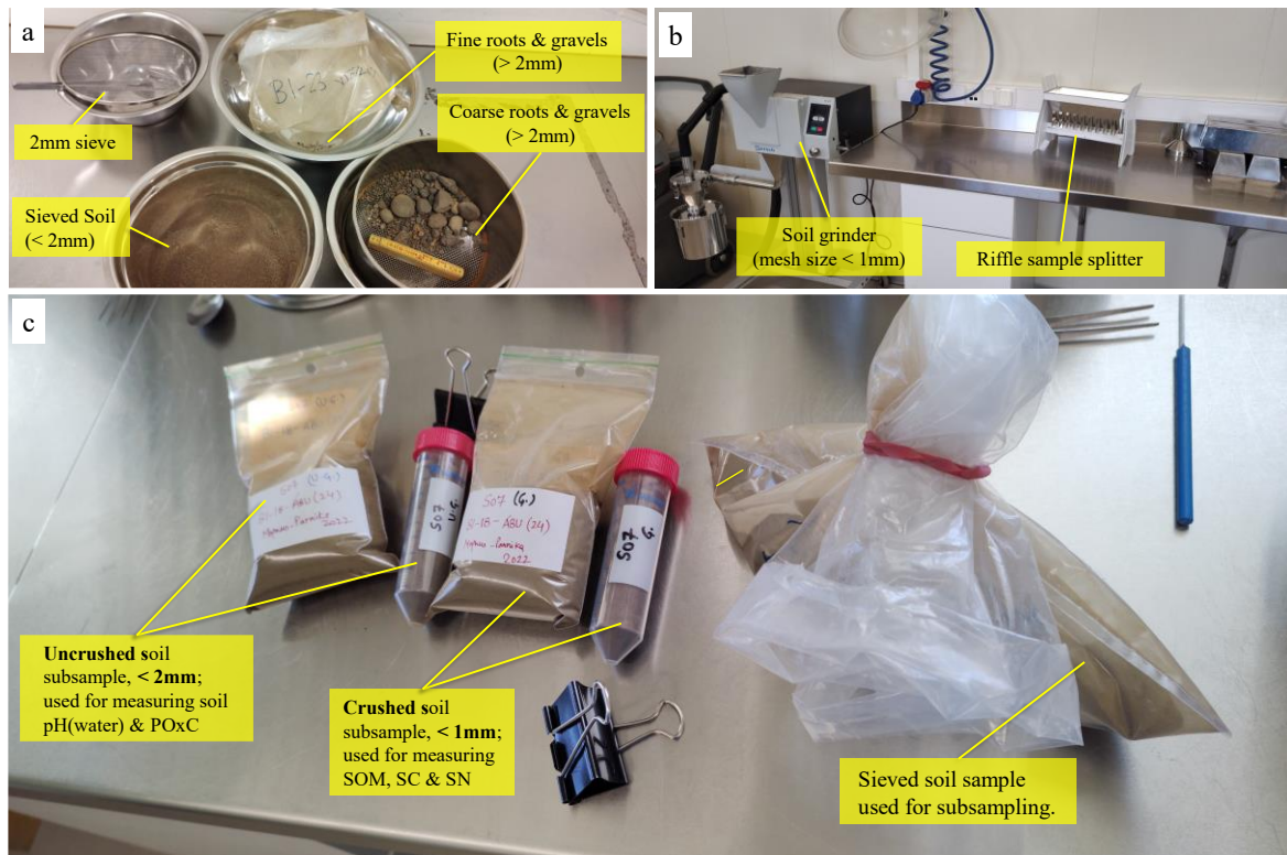
Figure 2.6 Soil sample preparation. (a) Soil sieving, (b) Soil subsampling setup, and (c) Soil subsamples: crushed (<1mm), & uncrushed (<2mm) (Photos by Parnika Gupta, 2022).
