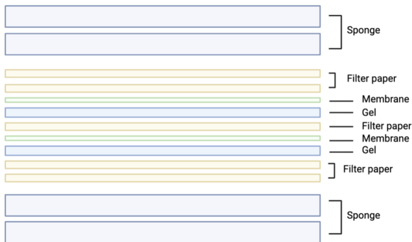
Figure 7: Showing sandwich setup for transfer of proteins onto membranes. Created with Biorender.com
